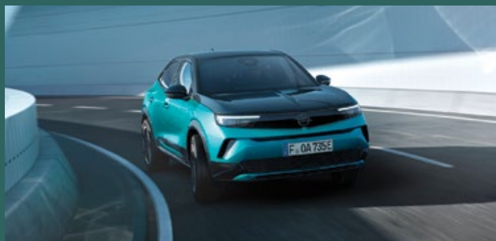
The new-generation Mokka Electric joins its petrol and hybrid siblings to complete the Mokka powertrain portfolio in Ireland. Sporting a 115kW 156hp electric motor and 54 kWh battery, the new Mokka Electric delivers up to 403km WLTP.
