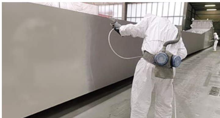
Spray painting the leg of a large ship to shore container crane
